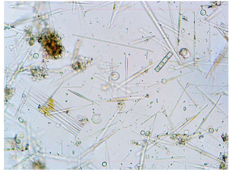
Figure 17: Diatom algae removed from clogged drinking water filter
